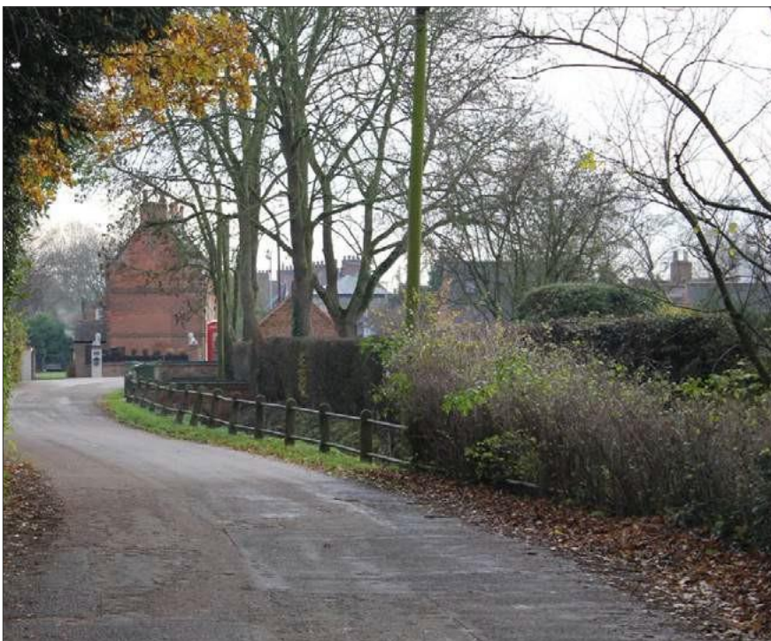
Streets for people: Minimal street clutter, lots of greenery and a surface treatment that encourages low vehicle speeds help make this street a place in its own right.
